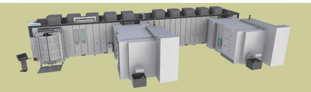
Mach Machine, Inc. recently expanded its automated production capabilities with the addition of two Okuma MB5000H attached to a 24-station Flexible Manufacturing System (FMS). This is a lights-out manufacturing system that operates unattended, day and night.
